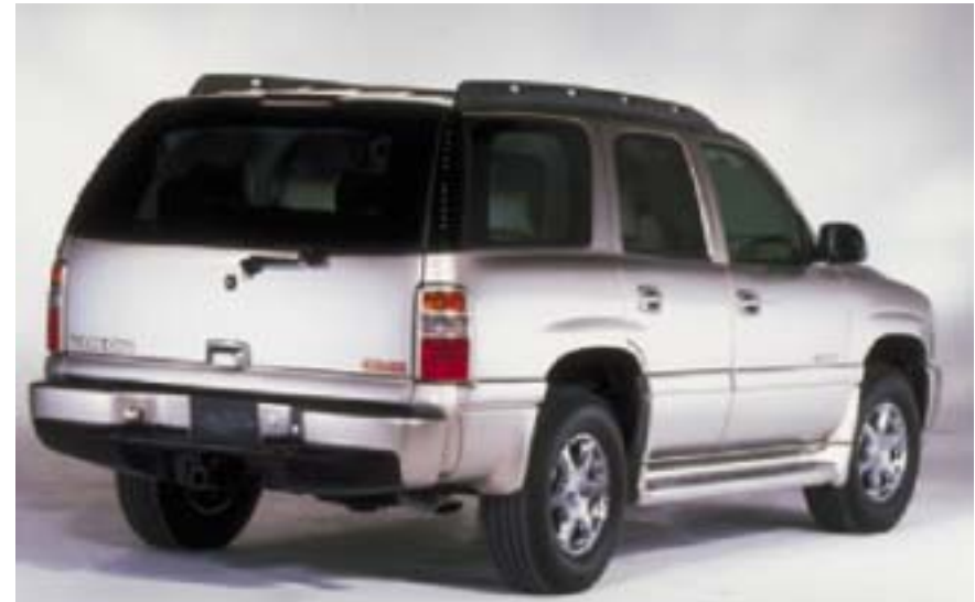
Aluminium spot welded liftgate on General Motors Yukon / Tahoe
