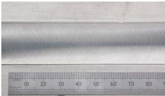
Fig 19 3 The surface of a typical tandem Twin-stir™ weld in 6082-T6 aluminium alloy 1 .
