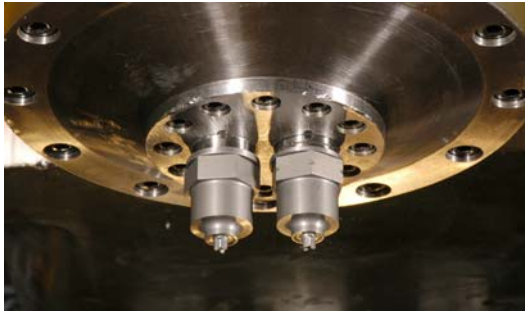
Fig 18 Twin-stir™ prototype head assembly 1 .
