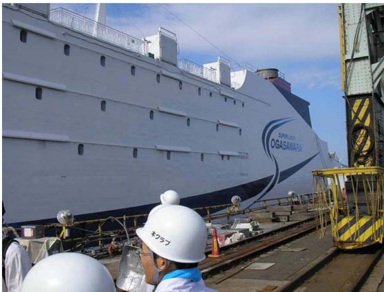
Fig 4. Aluminium ships constructed in Japan using FSW
