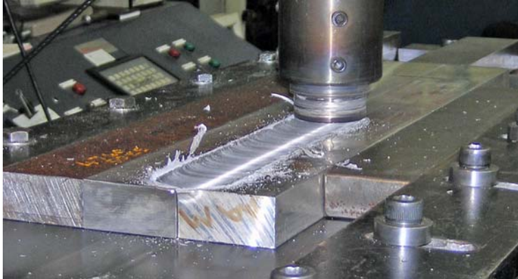
Fig 14 Welding 40mm thick 6082 aluminium alloy using a molybdenum probe.
