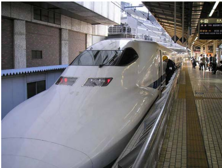
Fig 3. Japanese railway rolling stock fabricated from aluminium by FSW.
