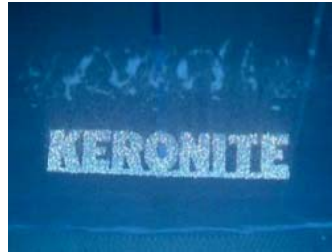
Plasma discharge in the electrolyte bath
