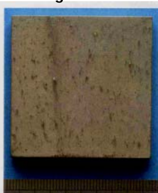
10 \mu m Anodised coating on AZ31
