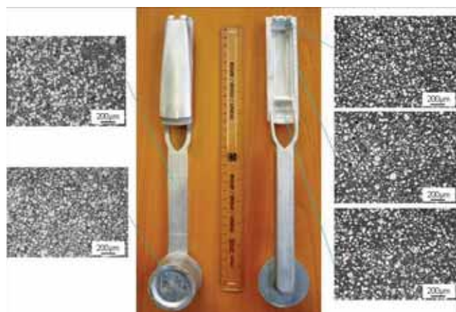
Fig 3: The first MC-TRC experiments using a conditioned melt of AZ91 have produced strip with a microstructure that is uniform across the whole width of the 4mm sample cross section
