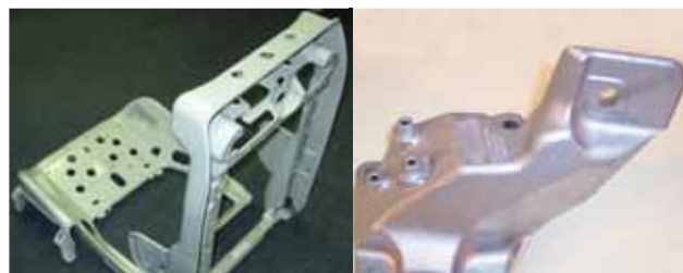
Fig 2: The new melt processors were used to high pressure diecast a magnesium seat frame and an aluminium engine mount
