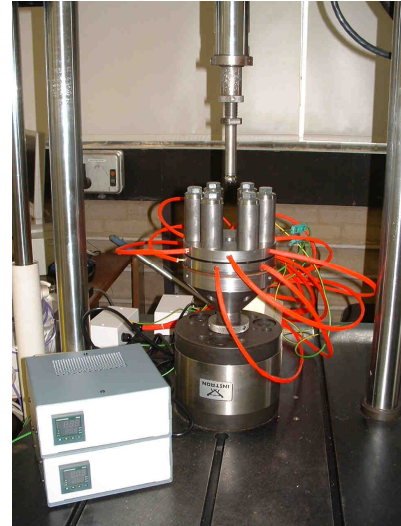
Figure 2 Heated tooling in load frame
