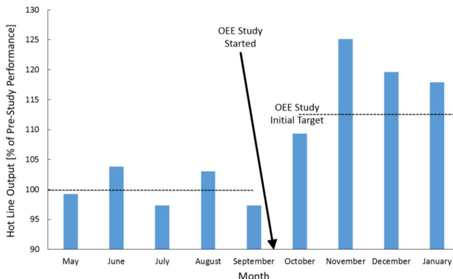
Figure 2: Plant data showing improvement in hot mill output following OEE study (performance normalised to 100% pre-study)
