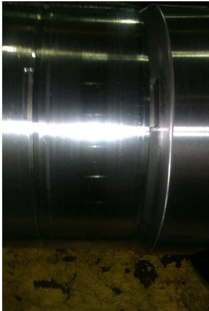
**Figure 2** Example of scratches on a roll bearing surface that can cause vibration chatter issues during rolling
