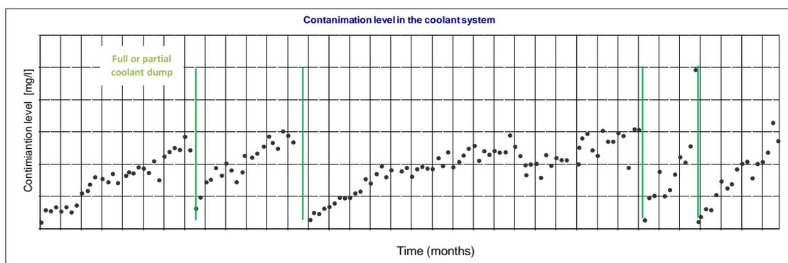
**Figure 3** Contamination levels due to an unidentified leak leading to poor performance and regular oil dumps
