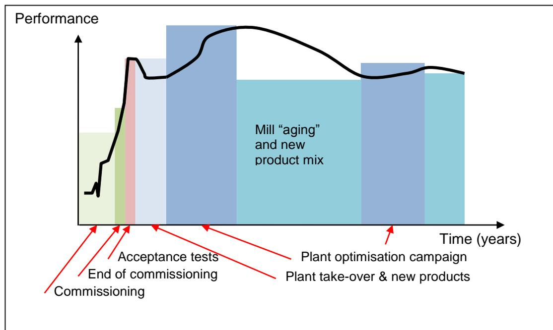
**Figure 1 Typical performance characteristic of a mill during its lifetime**
