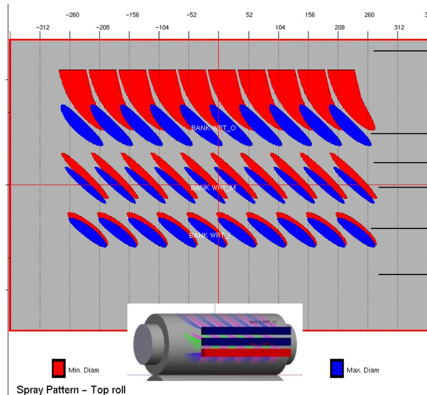
**Figure 4 Impact of a smaller work diameter on spray overlap**
