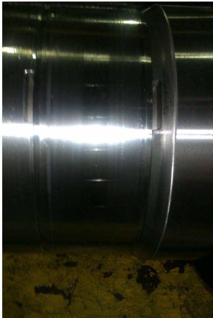
**Figure 3. Defects in work roll bearing inner races**
