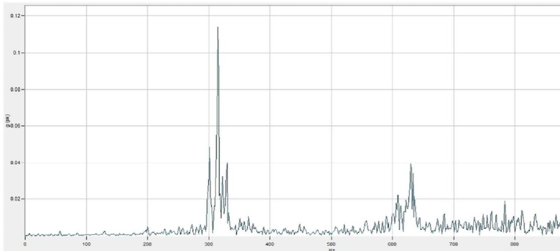
**Figure 1. Vibration spectrum from a work roll chock at 470 m/min showing forced vibration peak at 315 Hz**
