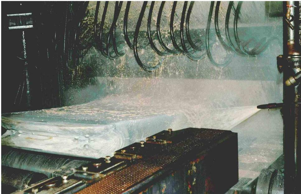
*Figure 2 - View of typical hot rolling mill showing lubricant application*
