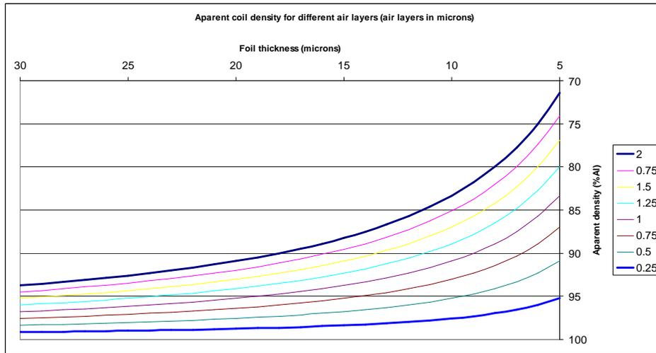
Figure 1. Relationship between coil density and gap between layers
