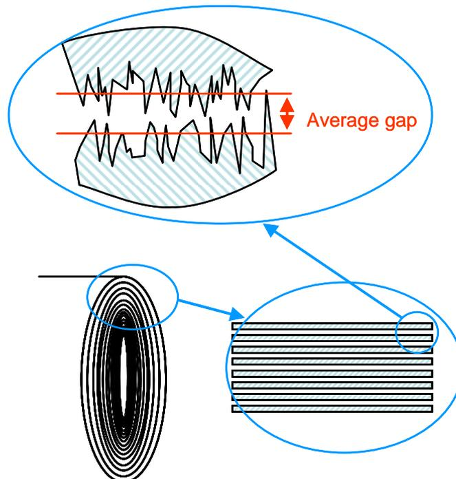
Figure 2. Schematics of gap
