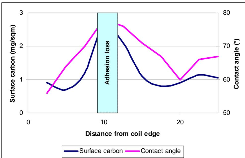
Figure 3. Relationship between carbon content on the surface and adhesion performance
