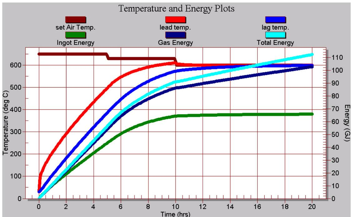
**Figure 6: Ingot leading and lagging temperature and energy consumed during a typical pre-heat cycle with higher initial set-air temperature**
