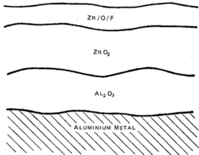
**Structure of zirconium based pretreatment**
