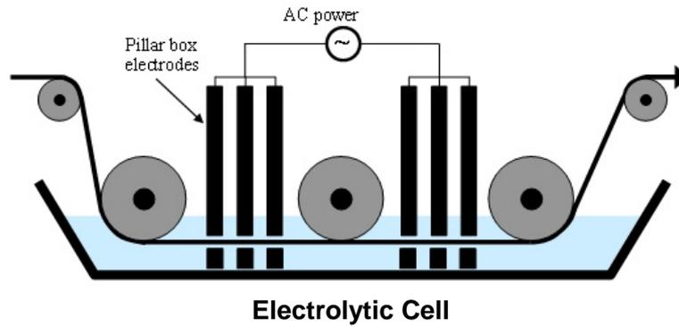
By using a.c., graphite electrodes, with slots through which the strip passes, can be used, pretreating each side of the strip simultaneously. The pretreatment film is produced whilst the strip is subjected to the anodic half-cycle, and the film is modified by chemical attack during the cathodic half-cycle. Full pretreatment can be effected in approximately 3 seconds. When using d.c., either lead, or lead covered, electrodes must be used in the cathodic section.
