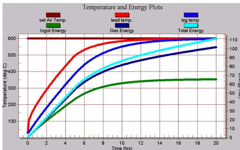
Figure 4 Ingot leading and lagging temperature and energy consumed during a typical pre-heat cycle with constant set-air temperature
