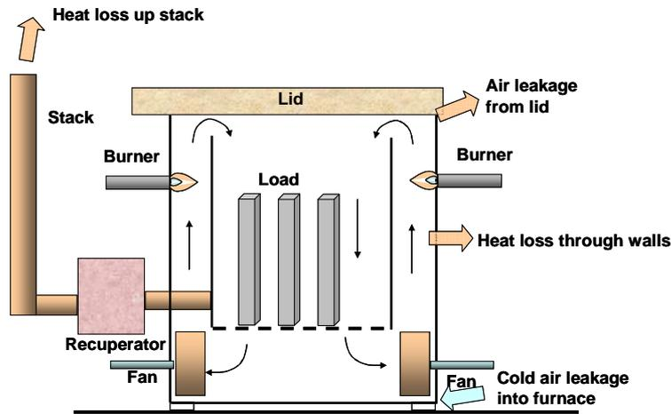
Figure 1 Schematic of a gas-fired pre-heat furnace
