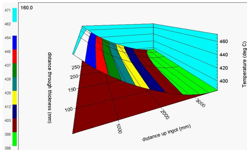
Figure 3 Temperature distribution in an ingot at mid-width position after 5 hours into the heating cycle
