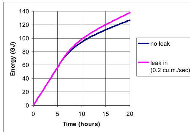
Figure 7 Effect on energy consumption of air leaking into a furnace
