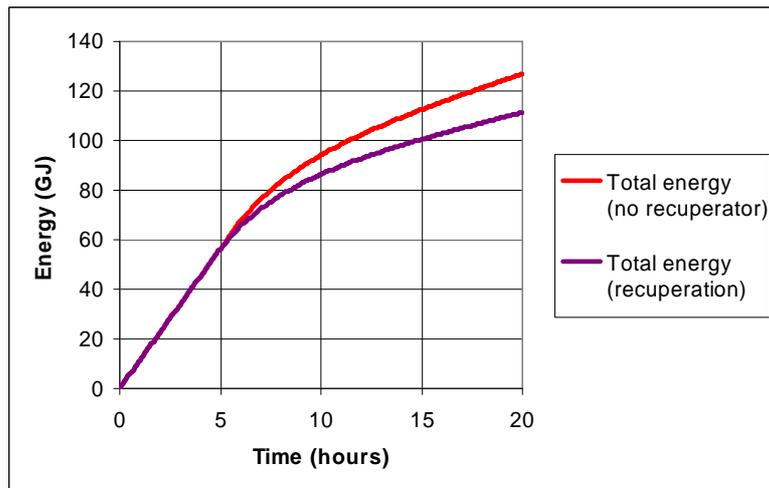
Figure 6 Effect of a recuperator on energy consumption
