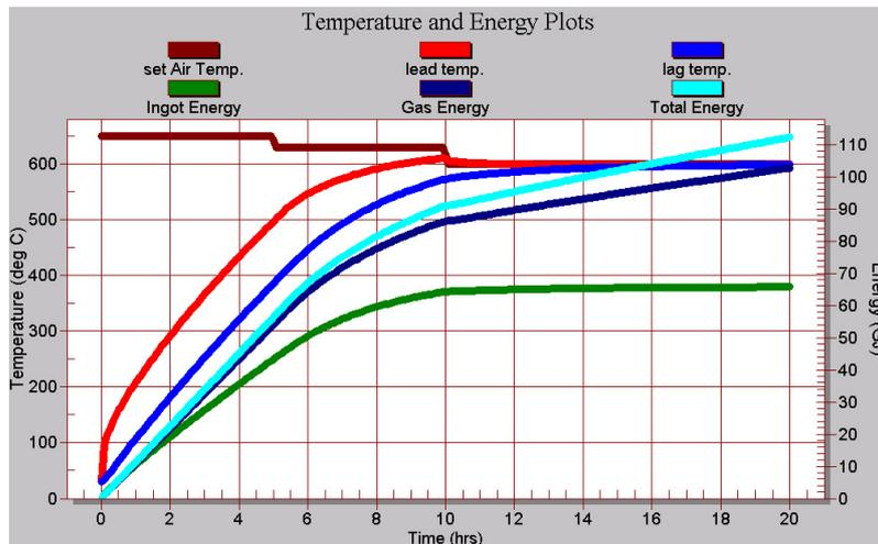
Figure 5 Ingot leading and lagging temperature and energy consumed during a typical pre-heat cycle with higher initial set-air temperature
