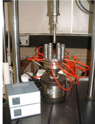
Figure 2 Heated tooling in load frame
