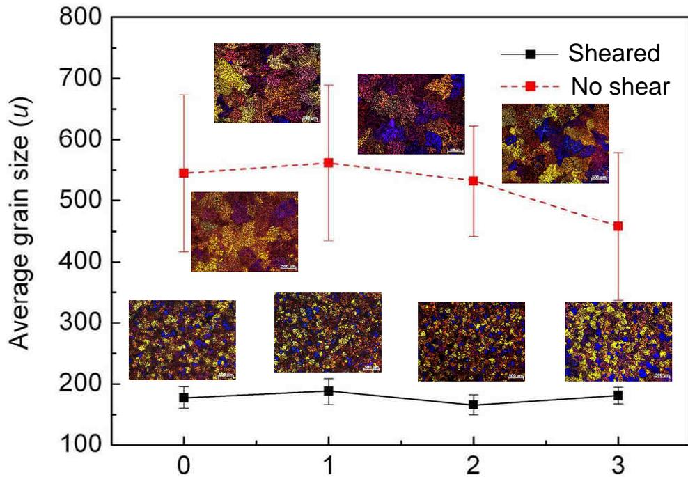
Figure 1: AZ91D cast with and without melt conditioning by the MCAST process at 650°C and then re-melted and cast three times
