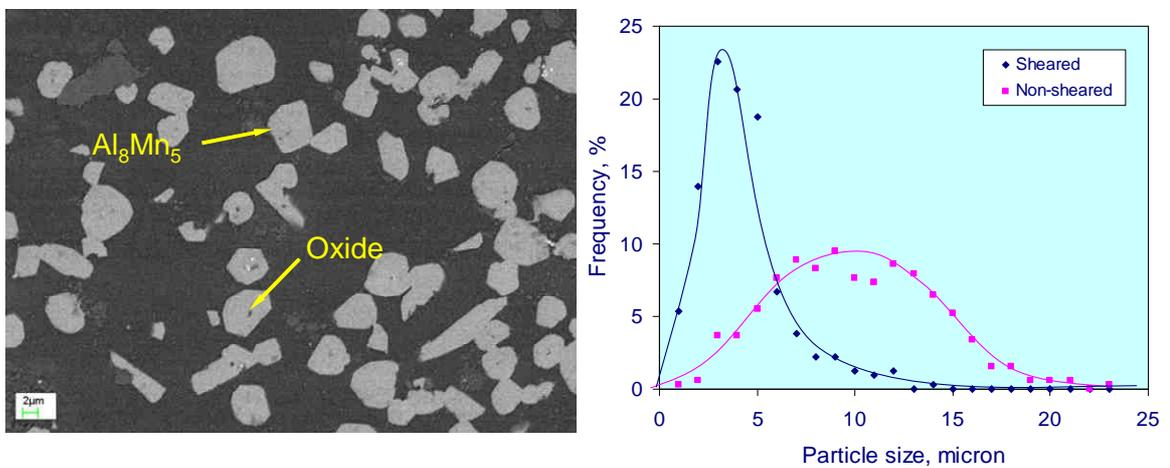
Figure 2: AZ91D filtrate after melt conditioning by the MCAST process showing the Al<sub>8</sub>Mn<sub>5</sub> intermetallics nucleated on dispersed oxide particles and the effect of melt conditioning on particle size distribution
