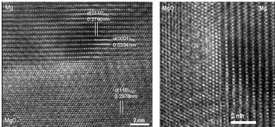
Figure 3: High resolution TEM images showing the close matching between the MgO and magnesium lattices
