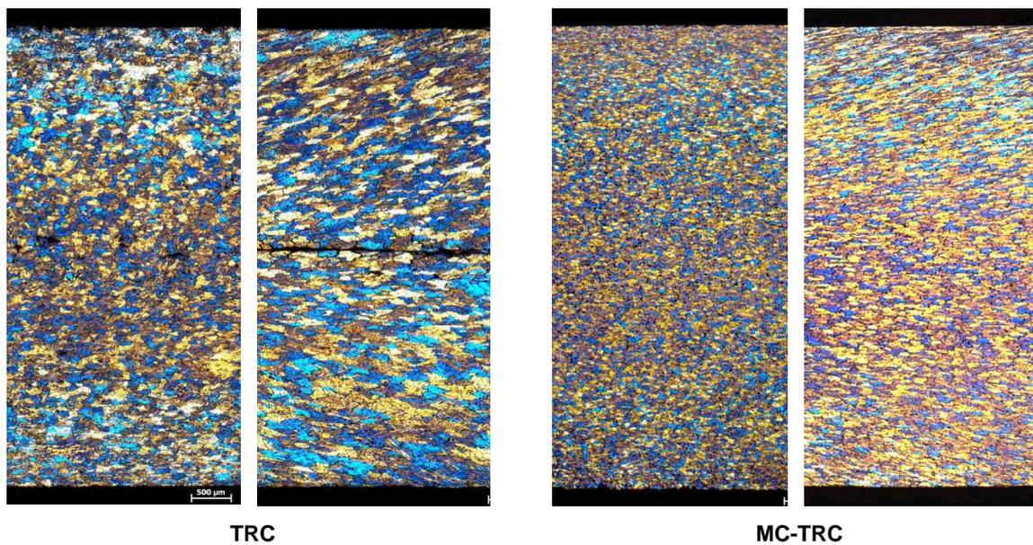
Figure 4: Comparison of grain structure and segregation in grain refined AA5754 (0.4 wt% Fe) twin roll cast with and without melt conditioning. (Longitudinal and transverse sections across the strip)
