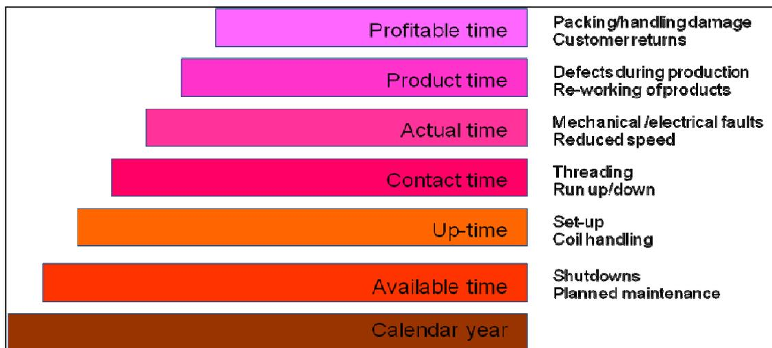
Figure 5. Attacking value through OEE mill studies
