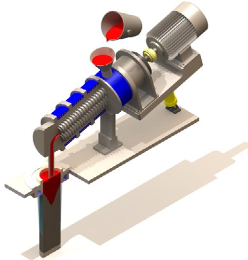
Figure 1: Schematic diagram of the twin-screw melt conditioner which forms the MCAST process
