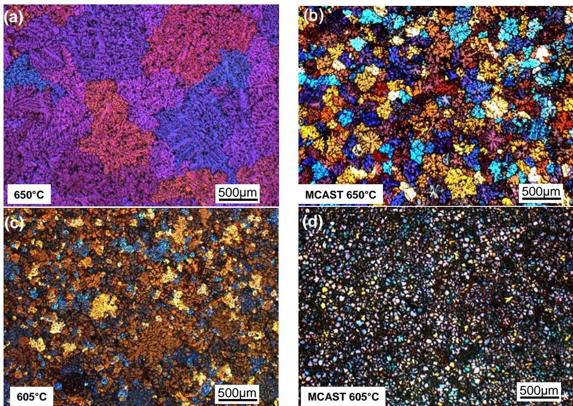
Fig. 2 Optical micrographs of typical microstructures of AZ91D castings showing the significant grain size reduction and after melt conditioning at 650°C (a) conventional, (b) MCAST and at 605°C (c) conventional, (d) MCAST
