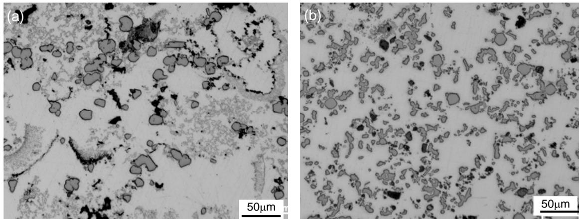
Figure 3: Optical micrographs showing the morphology of oxide and intermetallic Al<sub>8</sub>Mn<sub>5</sub> particles collected by pressurised filtration from (a) a conventional non-sheared melt and (b) a melt conditioned AZ91D alloy melt. Note the smaller particle size and the lack of oxide films in the conditioned melt
