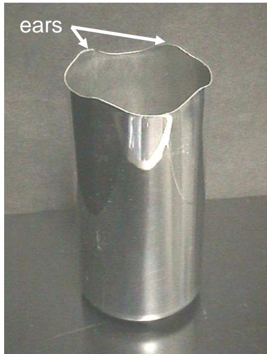
**Figure 2: Can after re-draw and wall ironing exhibiting severe “earring”**
