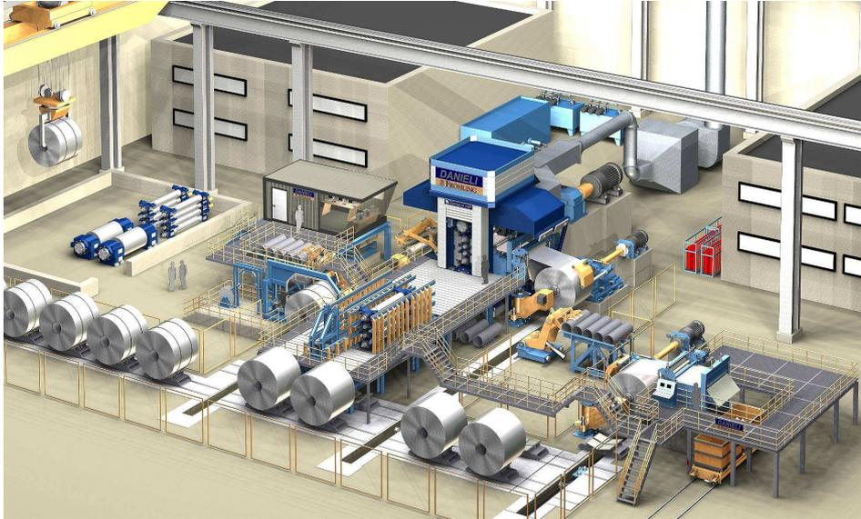
**Figure 3: Schematic showing layout surrounding a single stand cold rolling mill (courtesy of Danieli Fröhling)**
