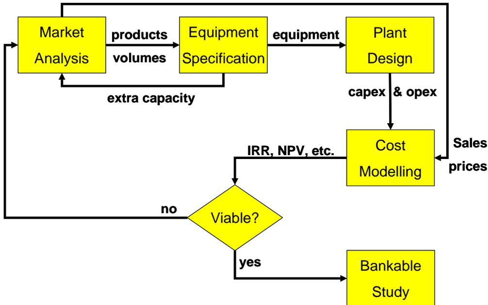
**Figure 1: Schematic flow diagram illustrating the main process steps in designing a successful and viable plant**
