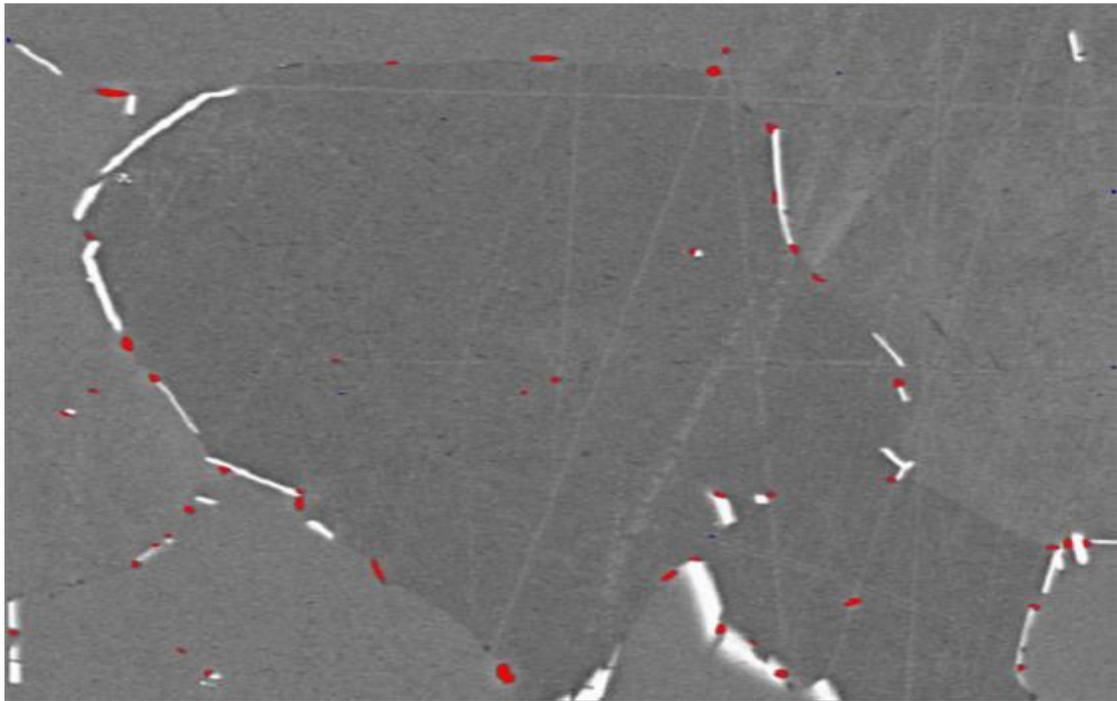
Figure 5: Micrograph showing Mg<sub>2</sub>Si (coloured red) and Fe-rich (white) intermetallics in billet.
