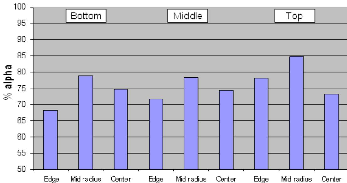
Figure 4: Variation in intermetallics through a homogenised 6063 log.
