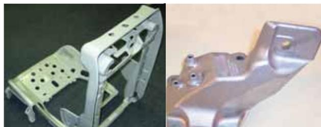
**Fig 2:** The new melt processors were used to high pressure diecast a magnesium seat frame and an aluminium engine mount
