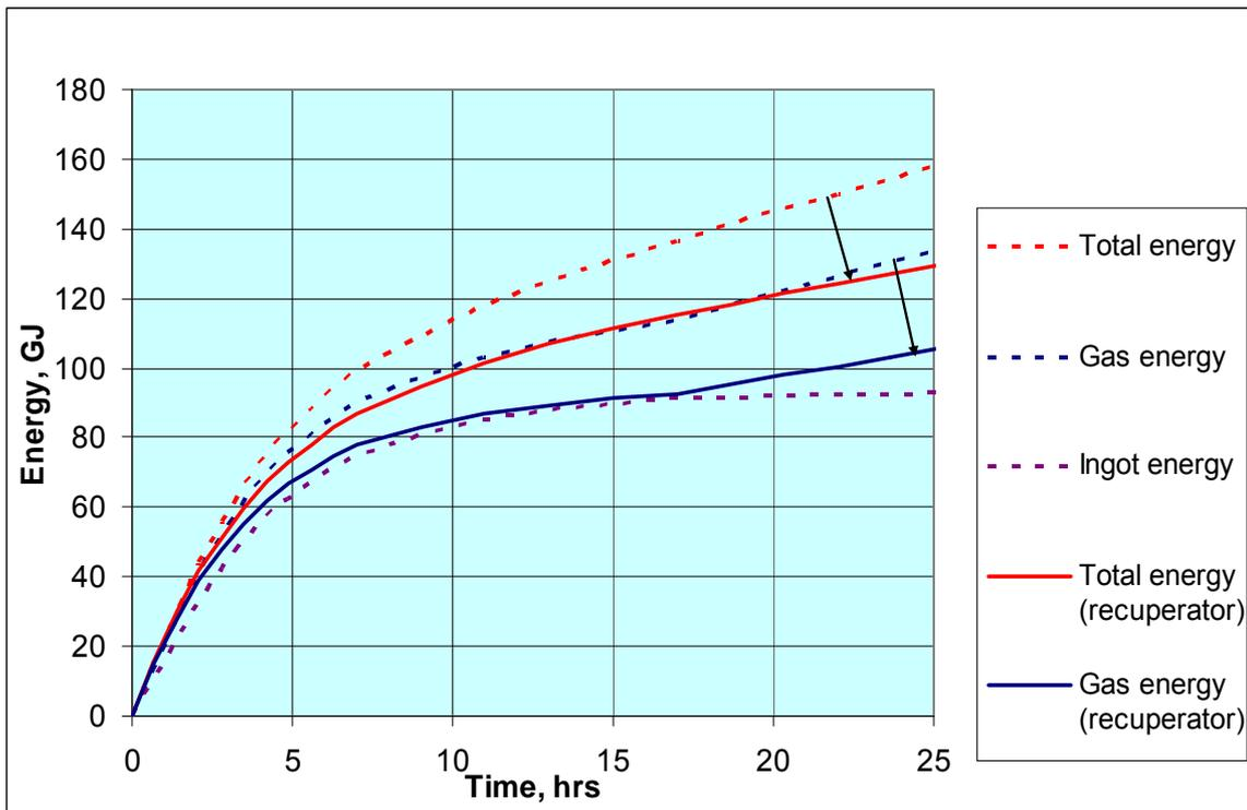
Figure 5 Effect of using a recuperator on the energies supplied.
