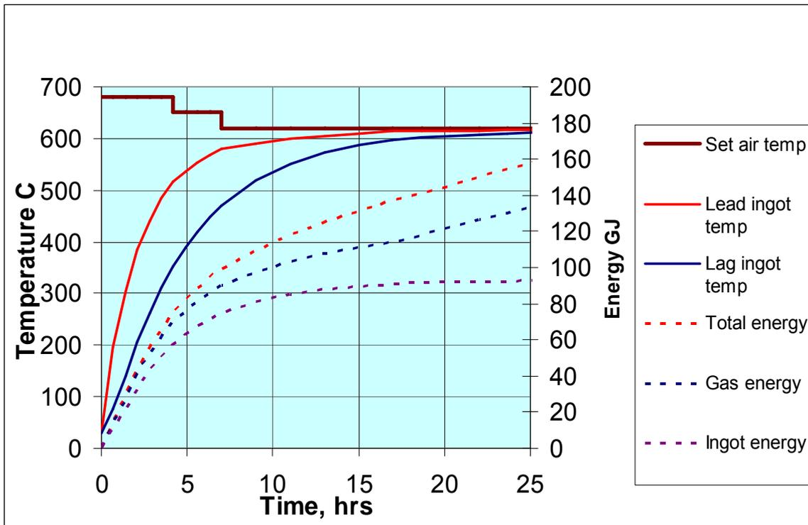
Figure 4 Leading and lagging temperatures in an ingot during the heat-up part of a pre-heat cycle. Also shown are the gas and electric energies supplied and the energy absorbed by the ingots.
