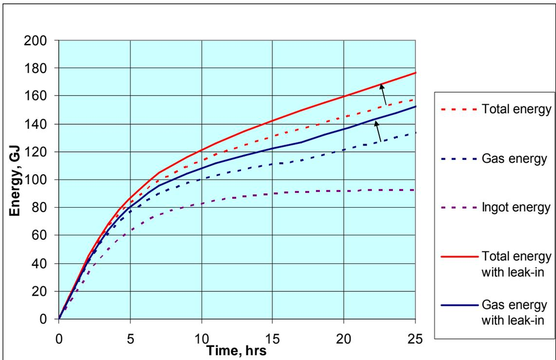
Figure 6 Effect on energies supplied of allowing 0.2 m³/s of cold air to leak into the furnace
