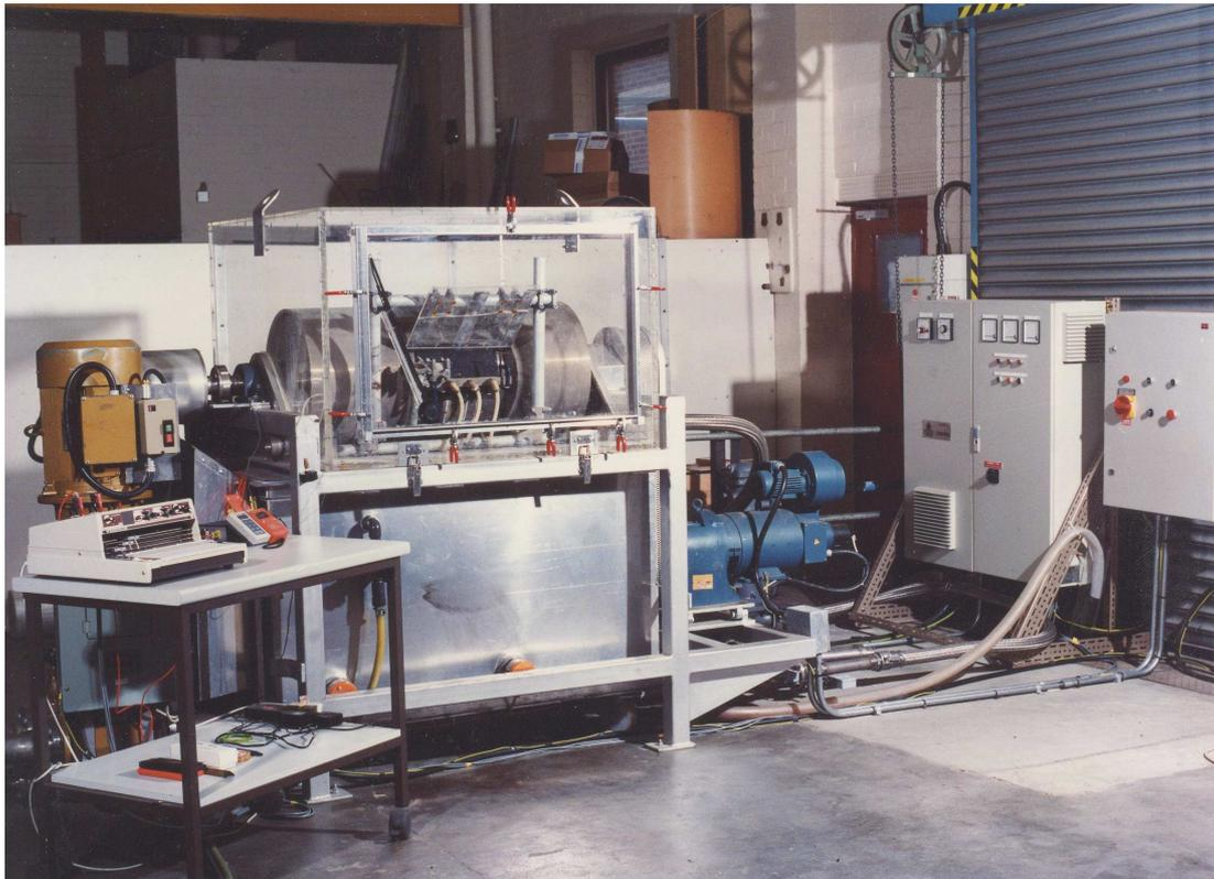
Figure 2 Test rig for measurement the heat transfer performance of cooling sprays (Reference 1).
