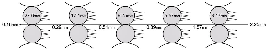
Figure 3 Schematic of a five stand tandem mill showing stand speeds and strip gauges.
