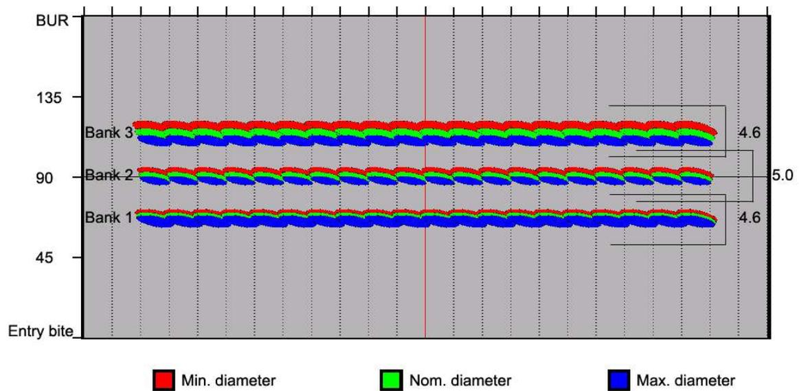
Figure 4 Spray patterns on the roll surface from three banks on the entry side of a mill stand. The figures to the right of each pattern are the calculated Cooling Effects of each bank (kW/K m width)
