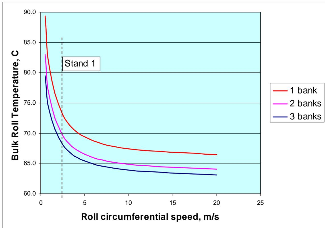
Figure 5 Effect of roll speed and spray distribution (one, two or three banks) on work roll temperature. The total coolant flow is the same in all three cases.
