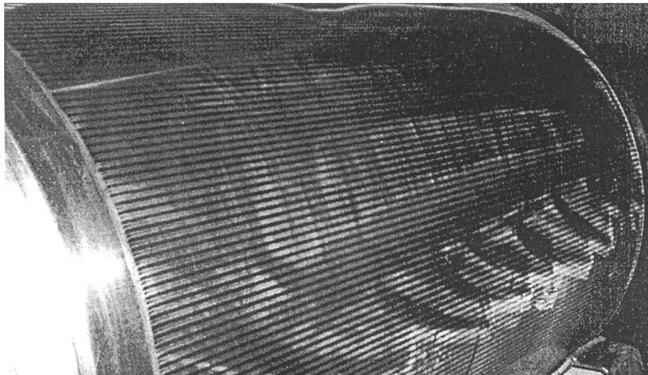
Figure 5: Example of severe fifth octave chatter marks on the barrel of a backup roll that would produce similar surface markings on the strip<sup>[4]</sup>.
