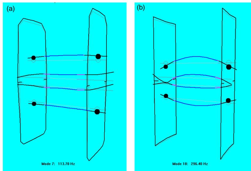
Figure 2: Typical mode shapes of rolling mill resonances that become excited during third octave gauge chatter. (a) shows the most common mode with a frequency between 100 and 150Hz and (b) shows a less common higher frequency mode. The lines represent the central axes of the rolls and housing frames in a 4-high mill<sup>[1]</sup>.
