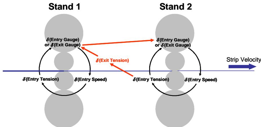
Figure 4: Interactions between two neighbouring stands in a tandem cold mill during mill vibration showing feedback of strip tension variation and feedforward of strip gauge variation.
