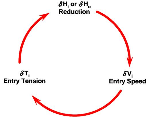
Figure 3: Mechanical feedback loop that exists in every mill stand with the potential to cause self-excited third octave gauge chatter.
