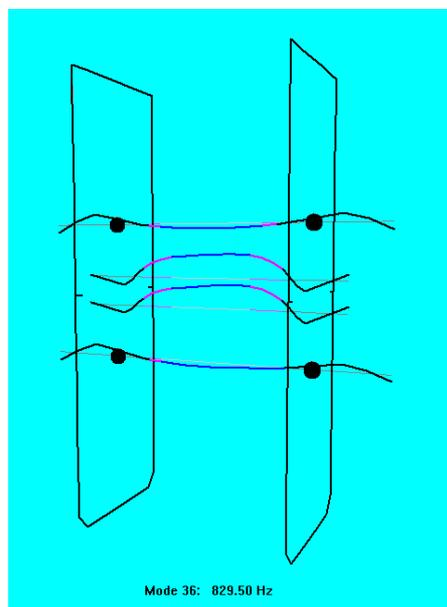
Figure 6: Typical mode shape of a rolling mill resonance that can become excited during fifth octave chatter. The lines represent the central axes of the rolls and housing frames in a 4-high mill<sup>[1]</sup>.
