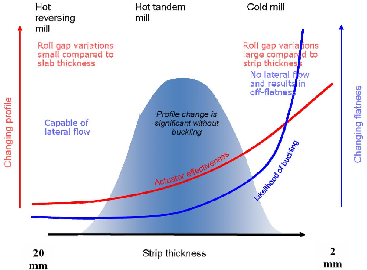
Figure 4 Dependencies on thickness of ability to change profile & likelihood of buckling
