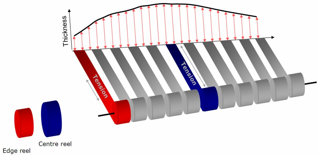
Figure 2 Impact of profile on multi-slit coils
