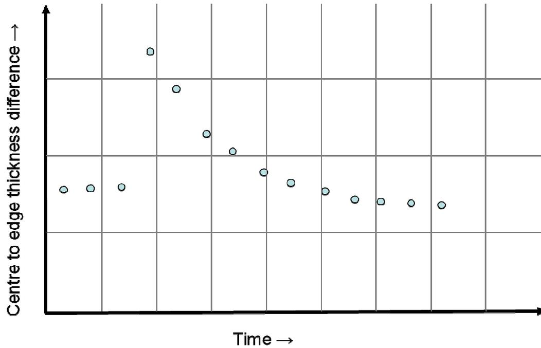
Figure 5 Transient in crown value caused by a product width change
