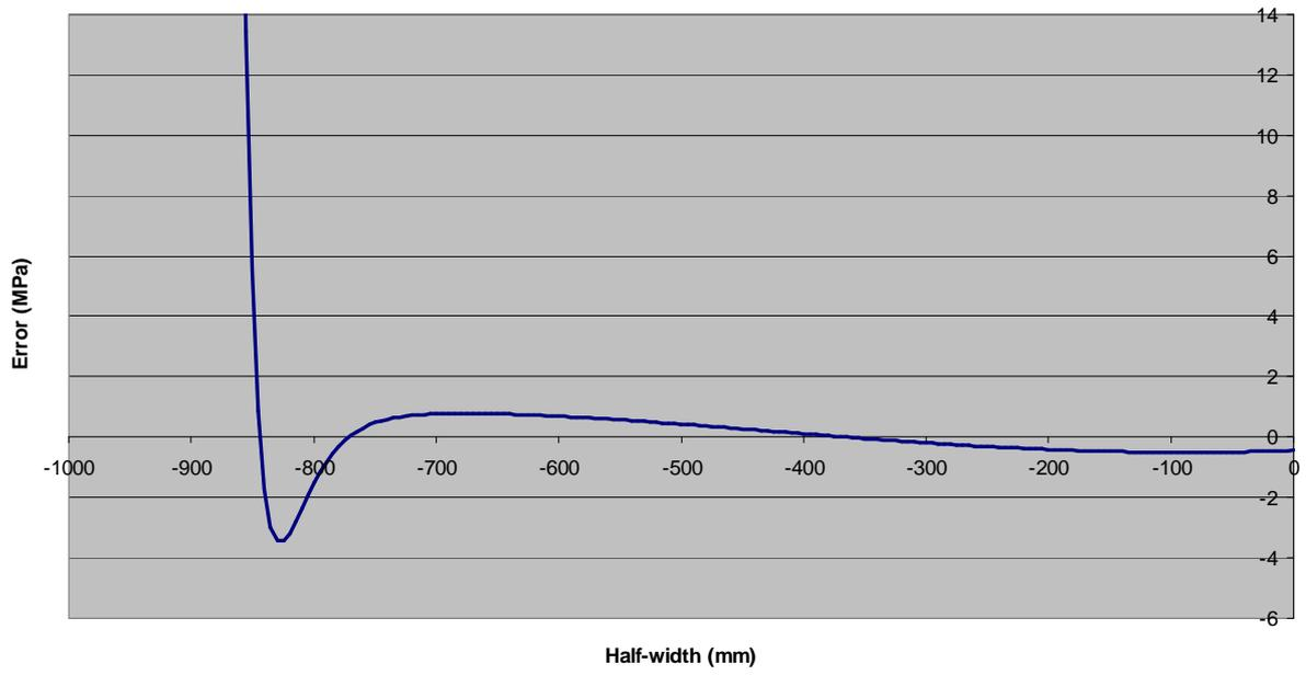
Figure 7 Typical flatness deviation from target (shown for only half the strip width)
