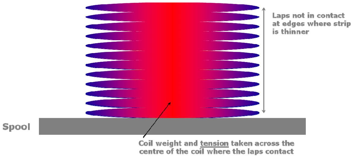
Figure 3 Schematic of how laps are built up while coiling
