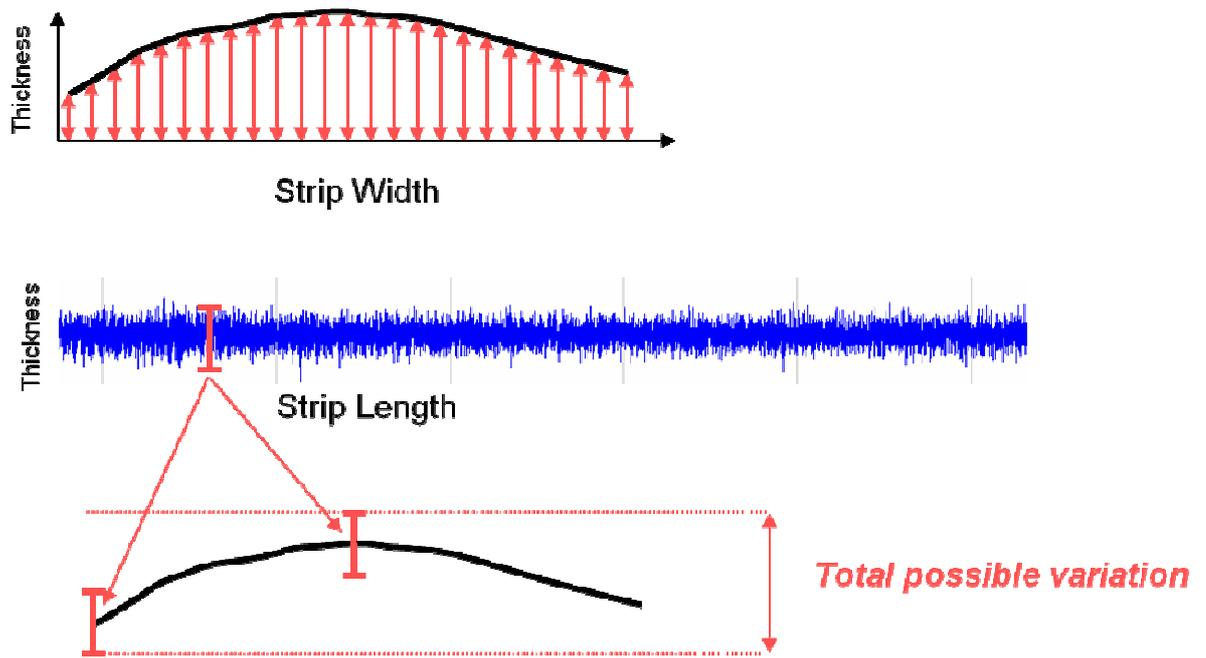
Figure 1 Makeup of total variation possible on coil thickness
