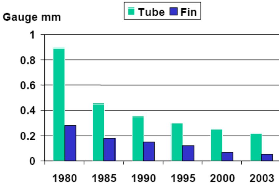
Figure 1 Downgauging trends in tube and finstock alloys
