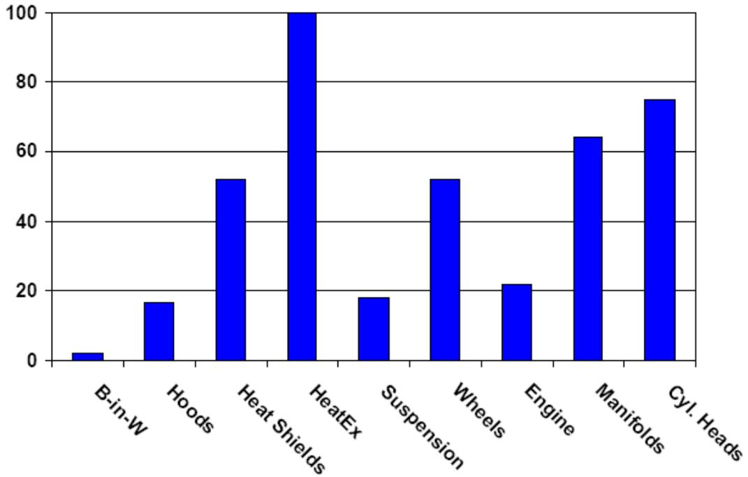
Figure 1 Aluminium Component Penetration % (US): source: Ducker Research
