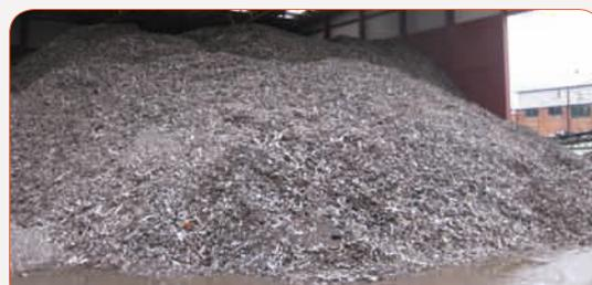
Zorba, the non-ferrous fraction of shredded cars
