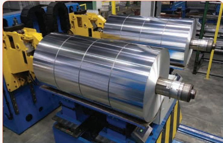
Coils of aluminium foil at the end of the separator
