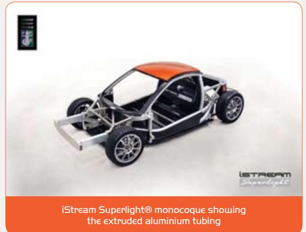
iStream Superlight® monocoque showing the extruded aluminium tubing
