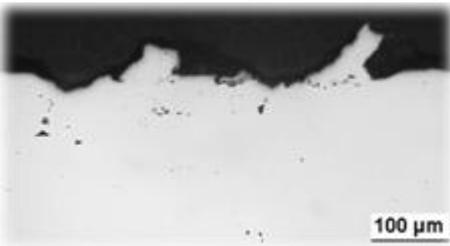
This image is of aluminium alloy AA7075-T651 taken from near the centre of the spherical projectile impact
