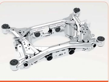
Jaguar I-Pace rear chassis fabrication consisting of aluminium extrusions, hydroformed tubes & pressings with fusion welding.
