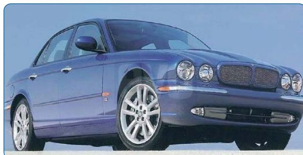
Jaguar XJ with Aluminium body and panels
