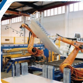
Robots lifting aluminium sheet at Novelis
