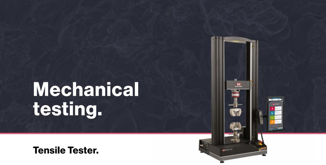
We've recently invested in a new Instron 50kN machine to enhance our materials testing capability. It allows us to perform a large range of accredited tests across a wide range of metals with very high accuracy.
